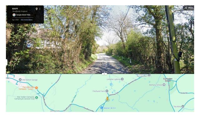
Install a beware pedestrians crossing sign on the bend, near to the two public rights of way – Pedestrian crossing signs are only for use on approach to formal crossings (i.e. zebra and signal controlled) but we could look to see if pedestrian in road signs, with distance plate, would be suitable. These could be installed on both approaches (subject to available verge) to the two PROWs
