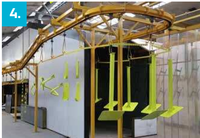
Painting Process – all parts are primed and powder coated in house through our paint plant.
